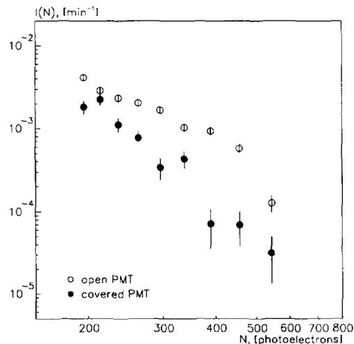
Figure 3. Amplitude spectra of detected events : open PMT – 4871 events, exposition 1510 min; covered PMT – 1613 events, exposition 956 min.
