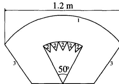
Figure 1. SPHERA optical scheme: 1 – mirror surface, 2 – PMT, 3 – diaphragm
