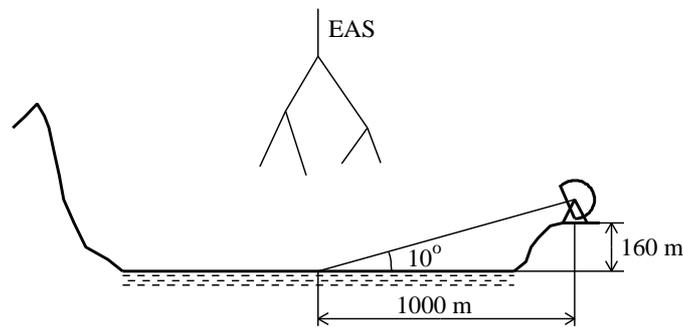
**FIGURE 3.** Geometry of experiment on B. Alma-Ata lake.
