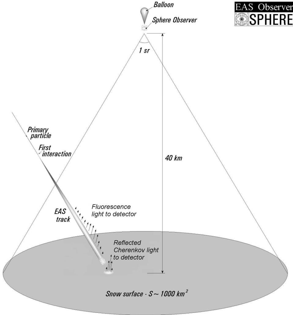
FIGURE 1. Geometry of the free balloon flight around the Pole.
