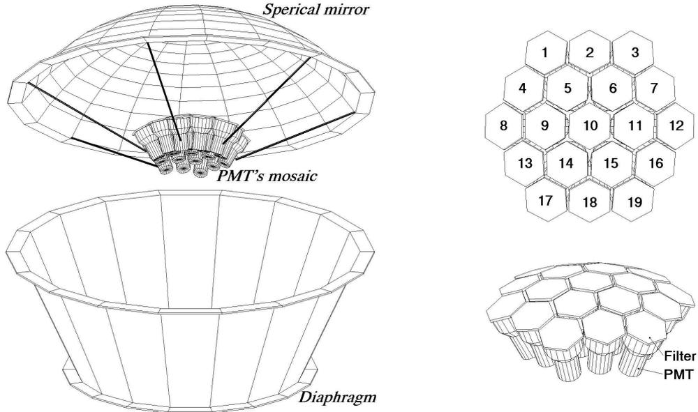
**FIGURE 2.** 3-D scheme of the optical part of the SPHERE detector.
