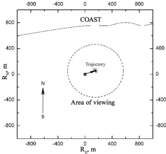
Figure 1. The layout of the experiment and the trajectory of flight of the tethered balloon according to GPS.
