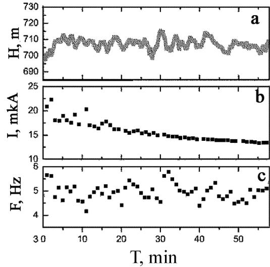
Figure 2. The information on equipment work. (a - installation height above the surface of Lake Baikal, b - an anode current for one PM in the mosaic, c - frequency of operation of the trigger)
