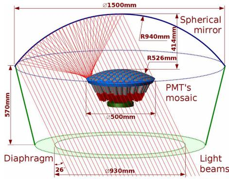
Figure 2: Optical scheme of SPHERE-2 detector.
