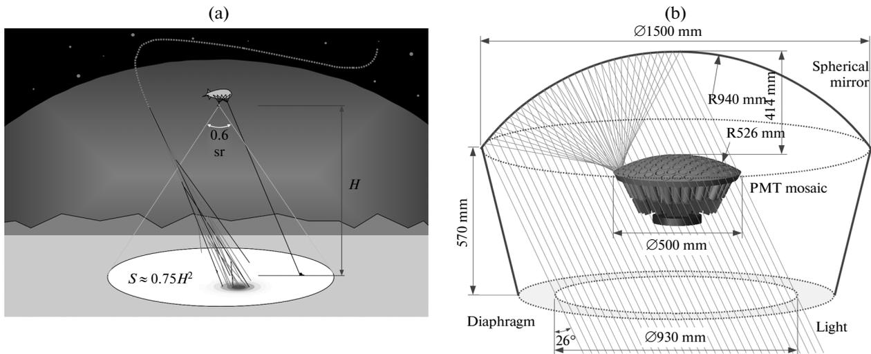
**Fig. 1.** (a) Design of the experiment performed on the ice of Lake Baikal using the SPHERE-2 facility; (b) optical scheme of the SPHERE-2 facility.
