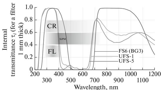
**Fig. 2.** Spectral characteristics of the FS6 (BG3), UFS-1, and UFS-5 optical filters. Horizontal bands denote the spectral regions of CR and FL and the region of SiPM sensitivity. The darker areas of the bands correspond to the radiation (sensitivity) maxima.
