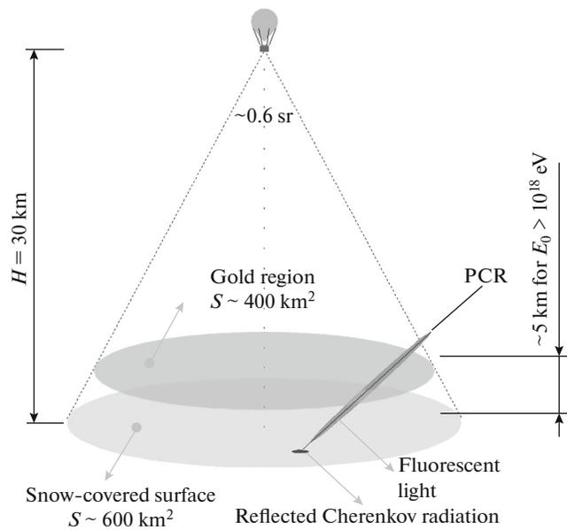
**Fig. 1.** Schematic diagram of the experiment in Antarctica. The SPHERE-Antarctica station and its prototype have similar geometric parameters, but differ in sensitivity and optical resolution (by a factor of ~10). Events from the gold region simultaneously contain data on CR and FL intensity.
