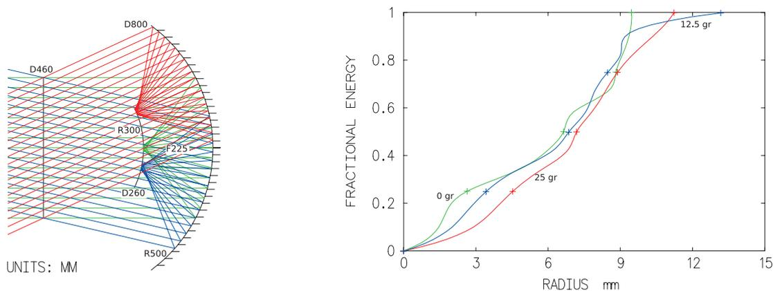
**Figure 3.** Optical scheme of the developed detector (without shadow from the mosaic) and the fractional light energy distribution on the focal plane taking into account the shadow from the mosaic. Red color corresponds to the rays coming at an angle of  $25^\circ$  from the optical axis, blue —  $12.5^\circ$  and green — paraxial.
