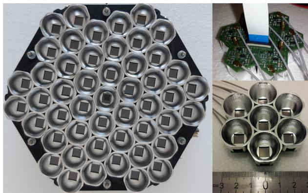
**Figure 5.** The prototype matrix of 49 SiPM assembled from seven electronic boards of 7 SiPM with preamplifiers.
