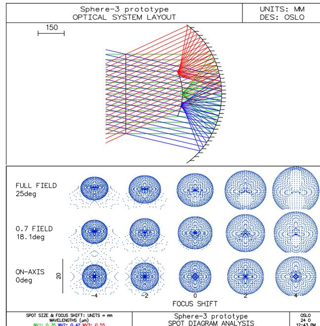
**Figure 2.** Preliminary version of the optical system with spot diagram analysis.
