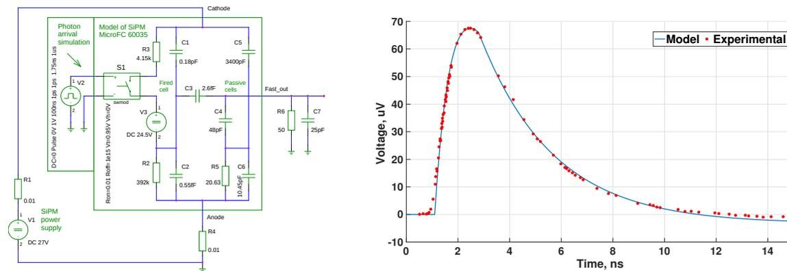
**Figure 3.** (Left) An electronic circuitry model approximating the real SiPM. The circuit model was built in MATLAB Simulink. (Right) The model curve of a current pulse from a single photoelectron obtained from MATLAB Simulink in comparison to the manufacturer provided data.
