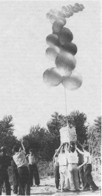
Fig. 1. Moment of launching the instrument for cosmic ray research on the garland of the balloons.
