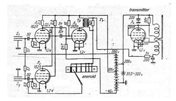
Fig.9. Electronic scheme of the experiment measuring cosmic rays on radiosond.
