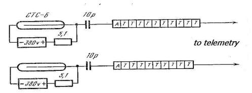
Fig. 2. Principal scheme of the detectors and of electronics placed onboard of the second Soviet satellite. A – amplifier of the signal from counter, T – trigger of the reducer of the count rate.
